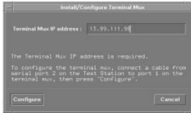
Figure 22 Terminal mux IP address entered into panel
